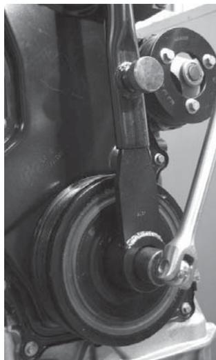
**AST4976 Crankshaft Pulley Holding Tool**
