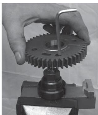
Remove the inlet camshaft gear from AST4978 Fixture ensuring that the Spacer Key remains in place in the gear window.
